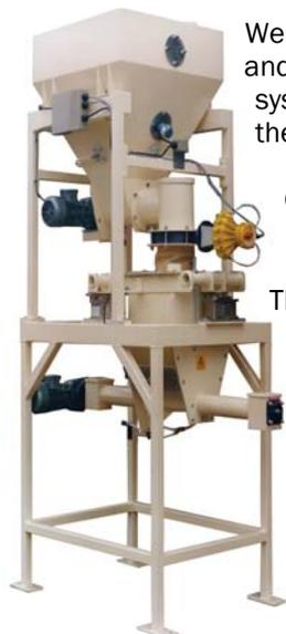
We have been working with the Loss-in-Weight concept for some decades now, and we have encountered and overcome most of the issues with this type of feeder. The example here shows a complete LIW sub-system complete with surge hopper, material conditioning and a special dual outlet. LIW is suitable for the most difficult of powders and even liquids.
