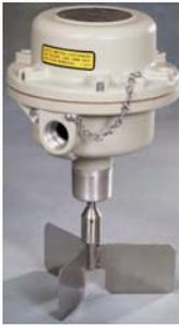
Unlike many other available paddle units Golconda's paddle level indicators incorporate a feature that automatically shuts off the motor of the unit when the paddle is in a stalled position, which both extends the life of the motor and minimizes maintenance.
